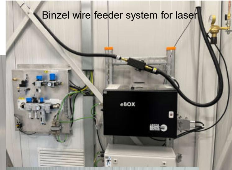
Binzel wire feeder system for laser
